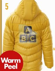
Remove the silicone sheet and peel away the clear transfer liner whilst the material is still warm.
