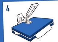
Using medium pressure press for 15 seconds at 160°C
