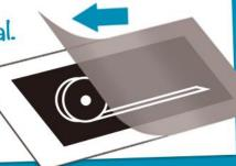
You should now have the graphic between both the paper release liner and the application tape.
