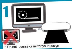
Cut your design using a plotter or contour cutter.
