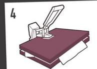
Using medium pressure press for 8-10 seconds at 140°C to 150°C
