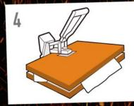
Using medium pressure press for 8-10 seconds at 140°C to 150°C
