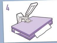
Using medium pressure press for 8-10 seconds at  $140^{\circ}\text{C}$  to  $150^{\circ}\text{C}$
