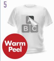
Remove the silicone sheet and peel away the clear transfer liner whilst the material is warm.
