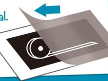
You should now have the graphic between both the paper release liner and the application tape.
