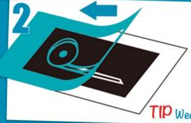
Once cut weed away the excess material until the finished design is left on the white release paper
