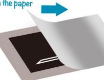
NOTE DO NOT try to lift the decal off the release liner using the application tape
